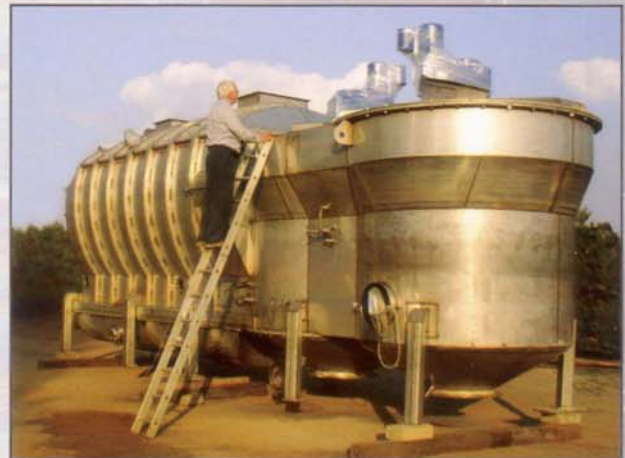
SF2M-1200 dryer for the sugar Factory Werbkowice S.A. (KSC Polski Cukier). Installation started up in 2005, capacity 50t/hr.
