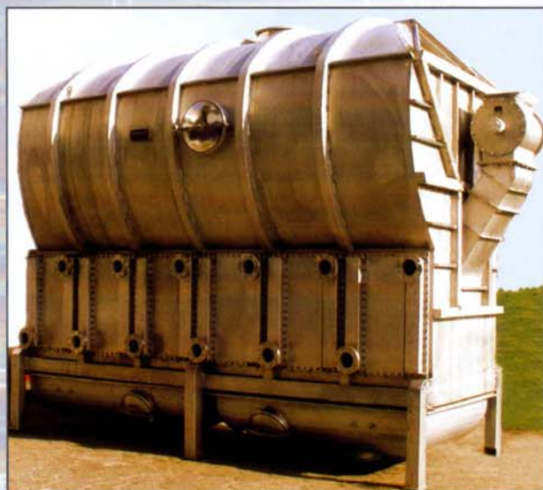
Fluid bed cooler with immersed heat exchanger.
