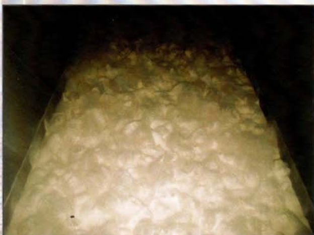
Fluidizing sugar in a fluid bed cooler, depth of the bed: 300mm.
