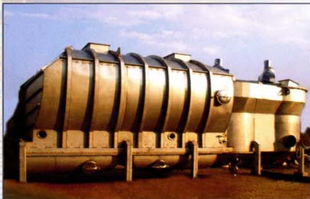
Fluid bed dryer for sugar with two rotating impellers, capacity 50 t/hr.
