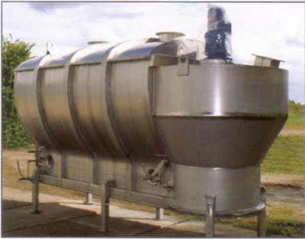
Fluid bed dryer for PET and ammonium sulfate manufactured for EKO-PET Ltd. in Kędzierzyn-Koźle.
